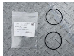
Replace PM10 inlet O-ring
