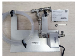
Replace Capillary for SO2
